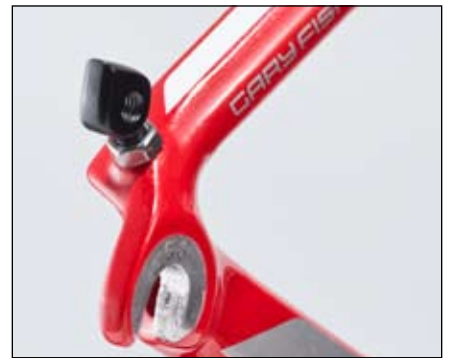
Figure 13. Eyelet with locknut installed in dropout
